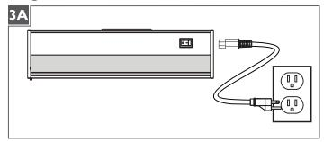
Using the Plug-In Wall Feed, plug the Undercabinet unit directly into a wall outlet.
