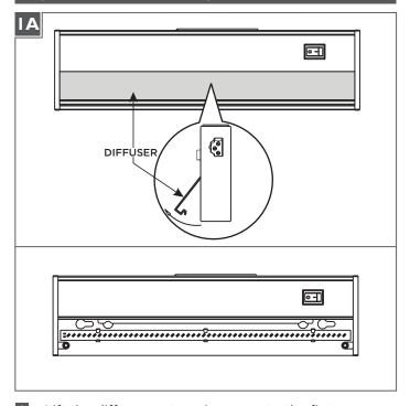
Lift the diffuser up to gain access to the fixture.
