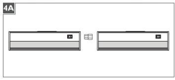
Remove the connector cover and use the Jumper Connectors to link multiple Undercabinet units to one another.
