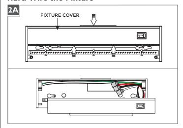
Remove the fixture cover by squeezing the inside of the cover to release it.
