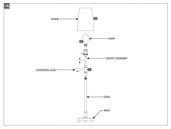
Adjust the height of the fixture by twisting the extension lock to loosen it and sliding the socket assembly into the desired configuration.
