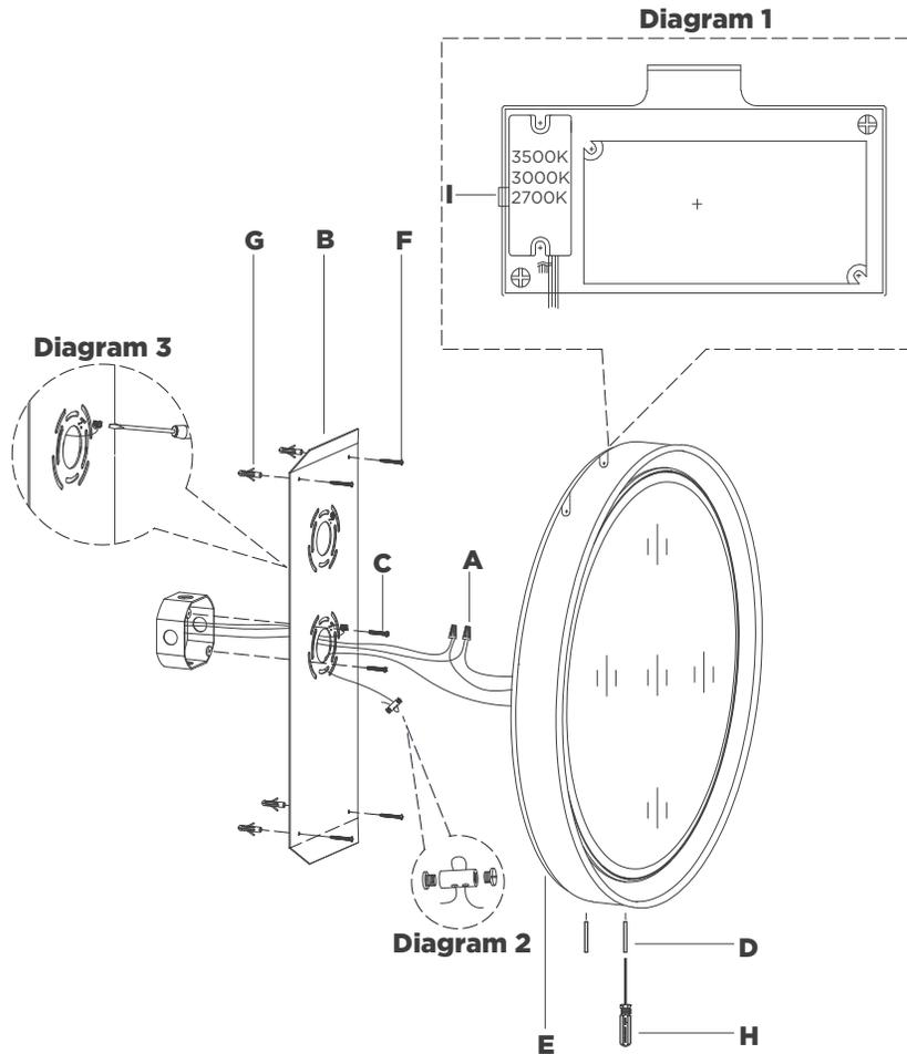
8. Connect fixture neutral wire (white) to the supply neutral wire (usually white) using wire nut **(A)**.
