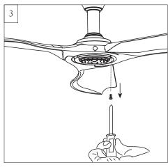
Remove LED light fixture by uninstalling the 3 set screws and turning counterclockwise.
