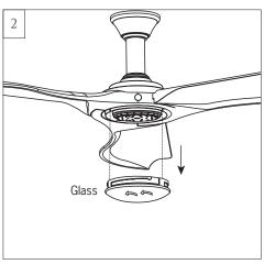
Remove glass from light pan by turning counterclockwise.
