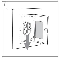
Before you begin handling light kit replacement, Switch power off at Service panel and lock service disconnecting means to prevent power from being switched on accidentally. When the service disconnecting means cannot be locked, securely fasten a warning device, such as a tag, to the service panel.
