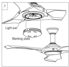
Attach blanking plate onto light pan by locating dimples in light pan with grooves in blanking plate and twist clockwise until tight.
