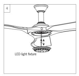
Disconnect the plug from fan and plug from LED light fixture.
