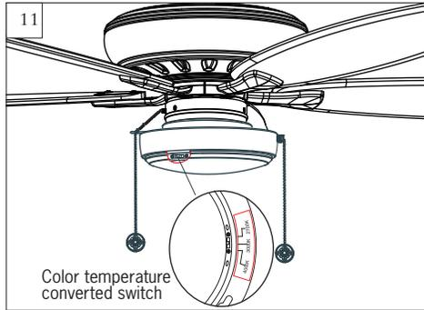
This light kit includes 2700 (Warm white), 3000 (Soft white) and 4000K (Daylight) correlated color temperatures (CCT). Get desired CCT by operating the converted switch.
