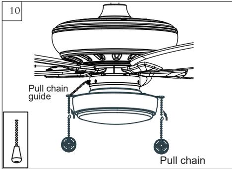
Install fan and light kit pull chains to preassembled pull chains on fan. Pull chains provided.
