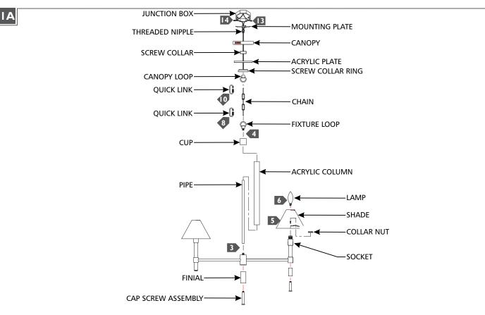
If necessary, screw the short end of the threaded nipple tightly onto the mounting plate, then screw the screw collar and canopy loop onto the threaded nipple.
