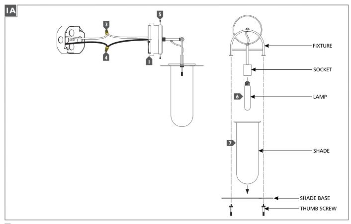
Secure the mounting plate to the junction box.
