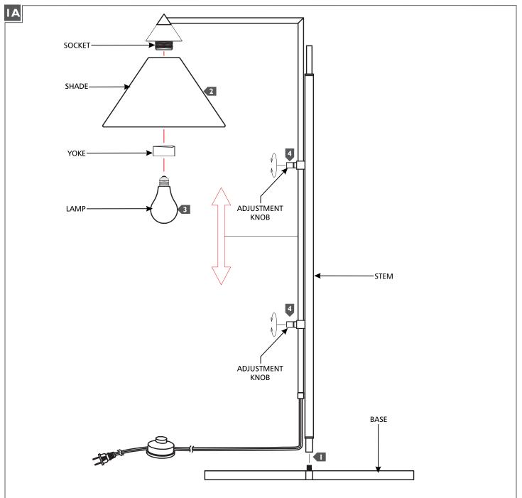
**I** Screw the base onto the stem.
