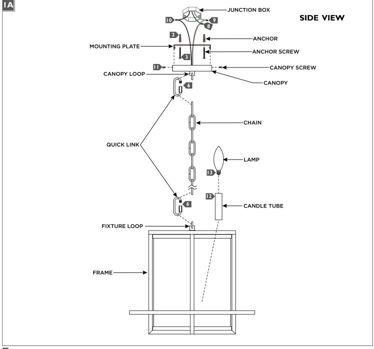
I Place the mounting plate against the ceiling mounting location and mark the anchor locations through the holes on the mounting plate. Remove the mounting plate from the ceiling.
