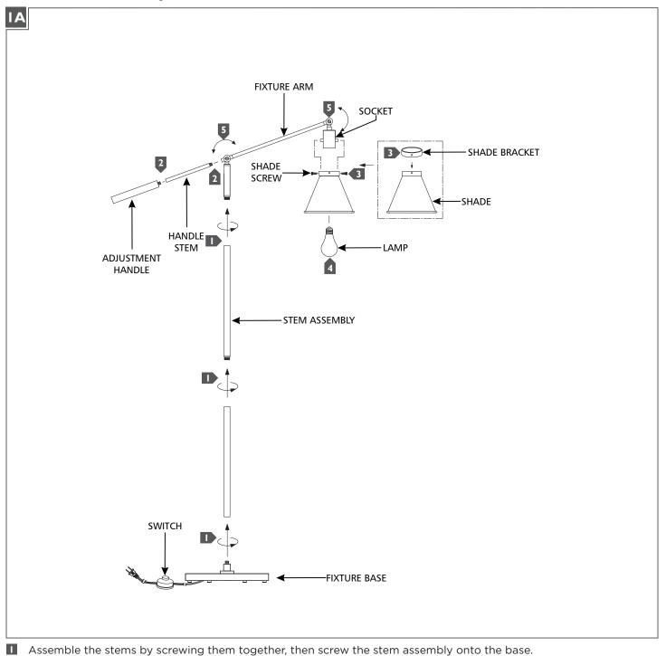
2 Screw the adjustment handle onto the handle stem, then screw the handle stem onto the fixture arm.
