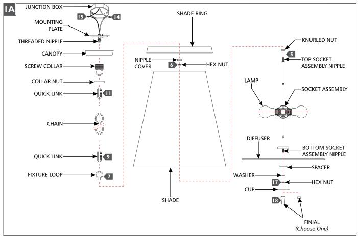
1 If necessary, screw the short end of the threaded nipple tightly onto the mounting plate.
