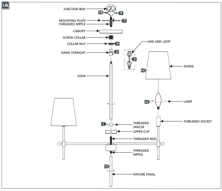
Feed the fixture wires through the top cup and spacer, and thread the spacer onto the threaded nipple.
