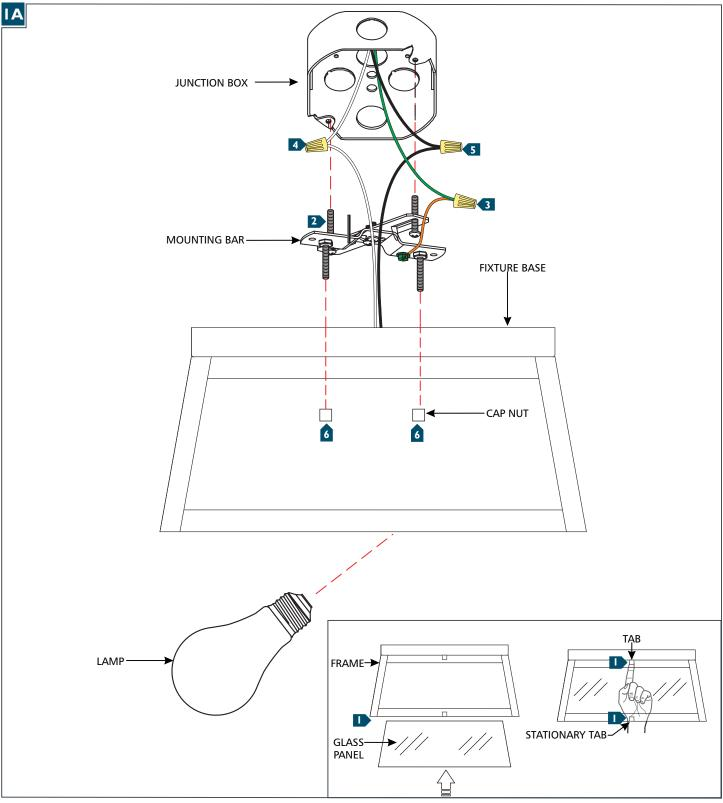
Install the glass one panel at a time into the frame by first inserting it into the bottom stationary tab, position the panel in place, then bend the top tab to secure the panels in place.
