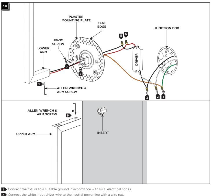
3 Connect the black input driver wire to the hot power line with a wire nut.
