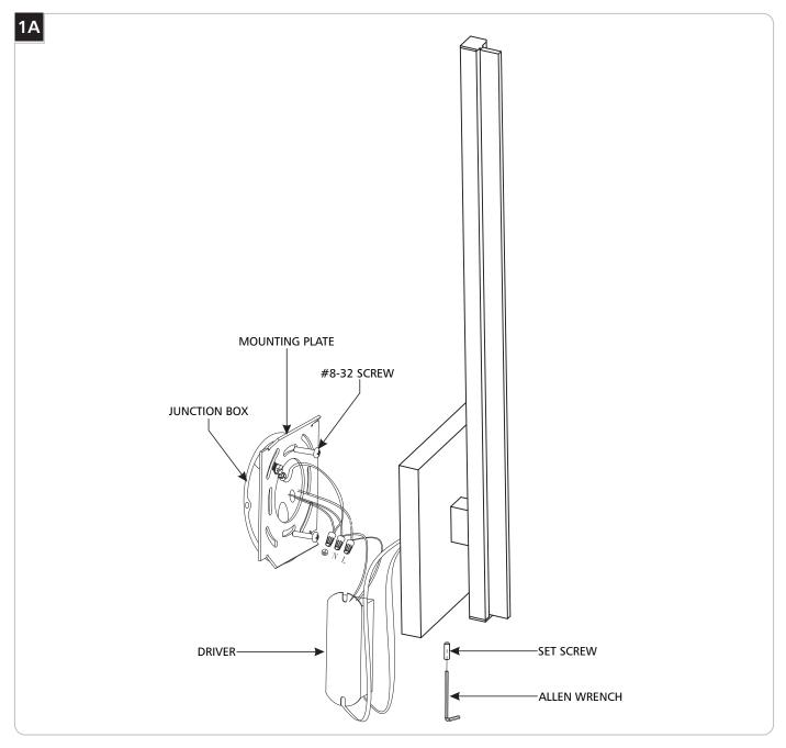
1 With the provided Allen wrench, remove the set screw on the bottom of the fixture base.
