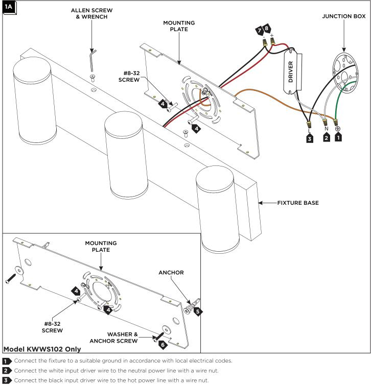
Properly place the driver/wire nut connections into the junction box and install the mounting plate to the junction box with the two provided #8-32 screws. For Model KWWS101, skip to step 7.
