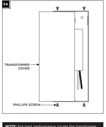
**NOTE:** For best performance, locate the transformer such that the length of the wiring between the transformer and the fixture does not exceed 500 feet.
