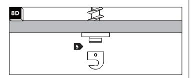
Hold the swag hook onto the washer and rotate it to the desired direction.
