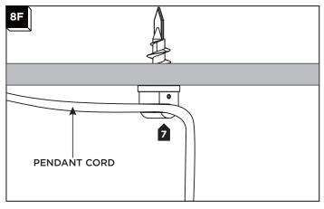
Hook the pendant cord into the swag hook and allow the pendant to hang freely.
