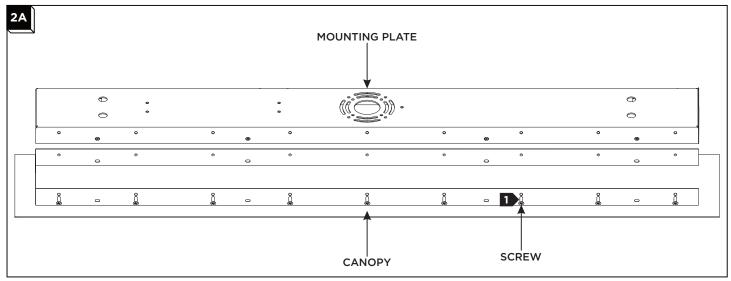
Remove the mounting plate from the canopy by removing the screws around the canopy.
