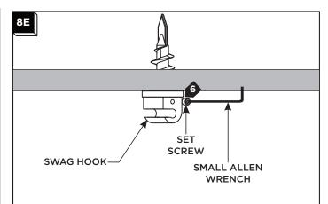
Secure the swag hook to the washer by tightening the set screw using the provided Allen wrench.
