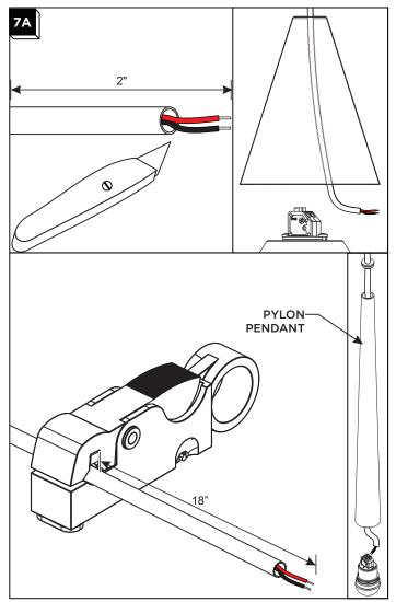
Measure the length of cord required to hang the pendant at the desired height and cut the cord. For Pylon Series, leave approximately 18" for internal wiring. For all other Head Series, leave approximately 2" extra length for internal wiring.
