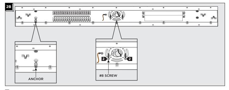
2 Secure the mounting plate to the junction box with the #8 screws provided
