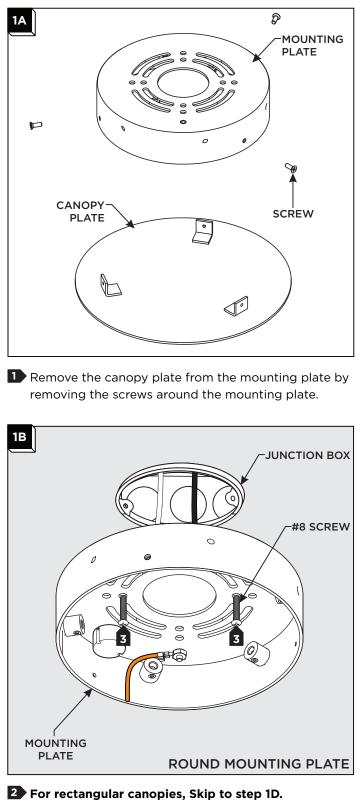
Secure the mounting plate to the junction box with the #8 screws provided. Reposition the drivers inside the canopy if necessary. **Skip to Step 2A.**
