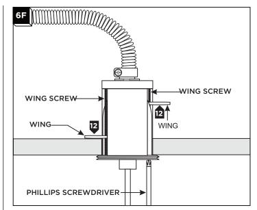
Tighten the two phillips screws with a Phillips screwdriver (an electrical screwdriver will speed up the process) until the wings secure the port into the hole.
