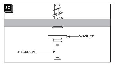
4 Mount the washer to the anchor with the #8 screw.
