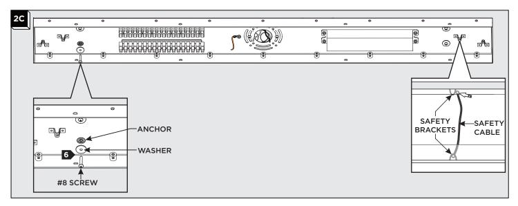
6 Slide a #8 screw through a washer and screw it into an anchor.
