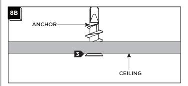
Screw the anchor in the rest of the way with a Phillips screwdriver.
