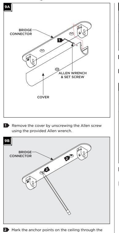
Mark the anchor points on the ceiling through the holes on the bridge connector near where the bridge connector is to be mounted.
