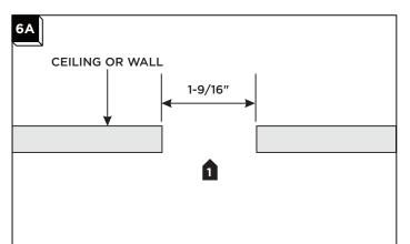
Use a 1-9/16" hole saw to cut out the ceiling or wall where the ports are going to be installed.
