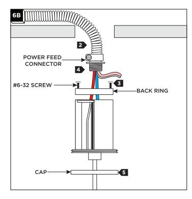
2 Bring the low-voltage wires to the ceiling opening.
