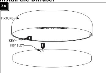
Alining the key slots on the diffuser to the keys on the fixture, slide the diffuser on then rotate it to lock in place.
