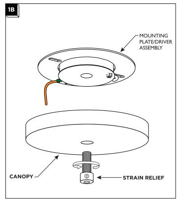
4 Remove the mounting plate/driver assembly from the canopy by completely unscrewing the strain relief.
