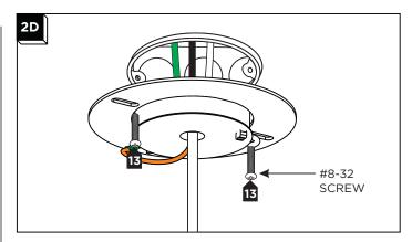
Properly place all wires and wire nut connections into the junction box and mount the mounting plate/driver assembly to the electrical box with the two provided #8-32 screws.
