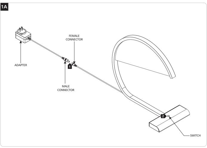
1 Connect the male connector from the adapter to the female adapter on the fixture.
