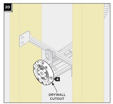
4 Install drywall to the joists and cut either the 2.75" diameter or 3" diameter size hole depending on the style of cover being used.
