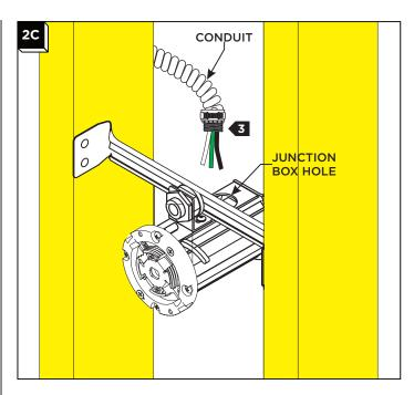
Attach conduit to either the top hole or the back plate of the junction box. Run wires for line voltage, ground, and dimming (if applicable) into the junction box.
