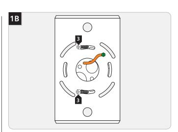
Attach the mounting plate to the electrical box using the two provided #8-32 screws .
