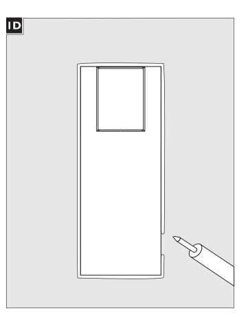
**For wet locations**, caulk around the base with waterproof construction sealant.
