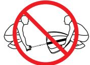
Warning: to avoid product damage, make sure to install the decorative fins after the chandelier body has been installed to the ceiling, as suggested by the following installation steps. Handling the fixture with the fins installed will cause damage to fixture.
