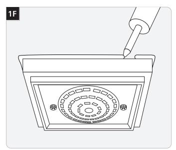
**10 For wet location installation,** caulk around the fixture base with waterproof construction sealant.
