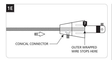
Feed and push the coaxial cable into the conical connector. The coaxial cable will come to a stop point after being inserted 3/4" into the conical connector.
