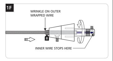
8 Keep pushing the coaxial cable into the connector while rotating the connector to ease feeding the inner wire into the tip of the connector. The outer wrapped wire will start wrinkling while being inserted another 1/2" into the connector.
