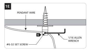
6 Hook the fixture pendant wire into the swag hook and tighten the #6-32 set screw snugly with 1/16 Allen wrench provided.
