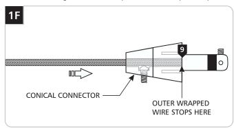
9 Feed and push the coaxial cable into the conical connector. The coaxial cable will come to a stop point after being inserted 3/4" into the conical connector.
