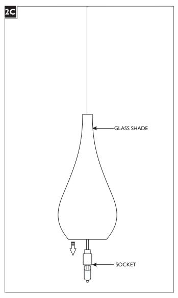
3 Lower the glass shade onto the socket assembly.
