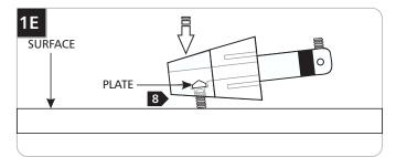
Tap the conical connector on a hard surface with the set screw facing down, so the plate inside drops into place.
