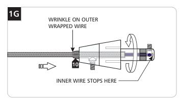
10 Keep pushing the coaxial cable into the connector while rotating the connector to ease feeding the inner wire into the tip of the connector. The outer wrapped wire will start wrinkling while being inserted another 1/2" into the connector.
