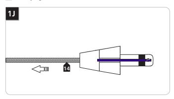
14 Pull the coaxial cable toward the fixture to smooth the wrinkles.
