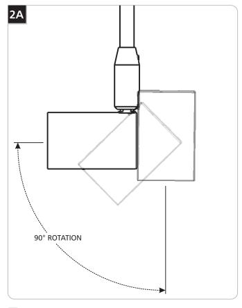
1 Rotate the socket up to 90°.
