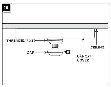
6 Place the canopy cover over the crossbar and screw the cap onto the threaded crossbar post.
