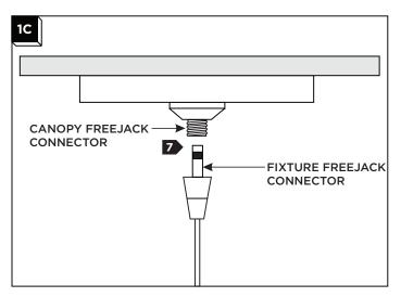
Screw the Fixture FreeJack male connector into the FreeJack female connector.
