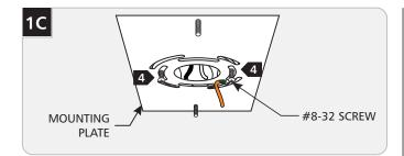
4 Secure the mounting plate to the electrical box with 2 #8-32 screws.
