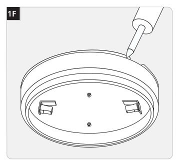
10 For wet location installation, caulk around the fixture base with waterproof construction sealant.
