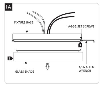
While supporting the glass shade, loosen (**Do Not Remove**) all the #6-32 set screws on fixture base with the 1/16 Allen wrench.
