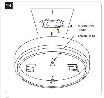
Remove the mounting plate from the assembly by unscrewing the two knurled nuts.
