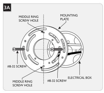
1 Align the two screw holes in the middle ring of the mounting plate vertically and secure it to the electrical box with the two #8-32 screws provided.
