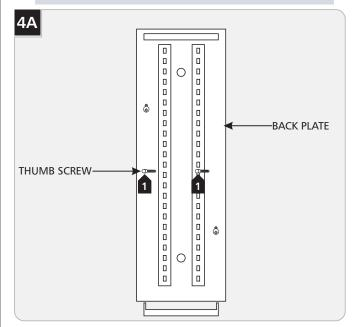
Temporarily mount the back plate onto the electrical box using the thumb screws, mark the anchor hole locations, and remove the fixture.
