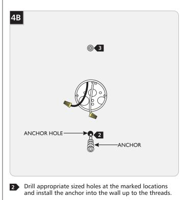
Screw the anchors in the rest of the way with a Phillips-3 head screwdriver.
