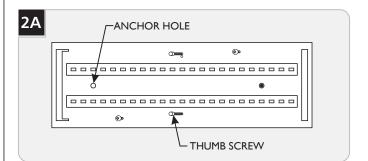
1 Temporarily mount the fixture onto the mounting plate using the thumb screws, mark the anchor hole locations, and remove the back plate.
