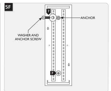
**1** Install washers onto the anchor screws, then fully secure the mounting plate by screwing the anchor screws into the anchors.
