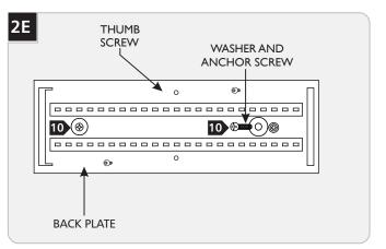
10 Install washers onto the anchor screws, then fully secure the back plate by screwing the anchor screws into the anchors.
