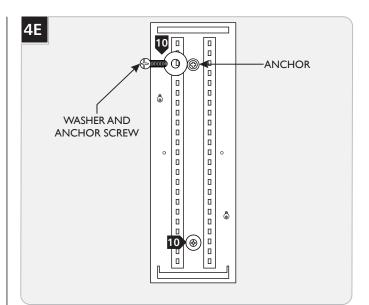
Install washers onto the anchor screws, then fully secure the mounting plate by screwing the anchor screws into the anchors.
