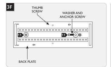
11 Install washers onto the anchor screws, then fully secure the back plate by screwing the anchor screws into the anchors.
