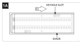
Remove the shade by sliding it all the way over to release it from the keyhole slot, then carefully pull it straight out.
