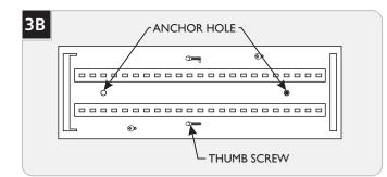
Temporarily mount the fixture onto the back plate using 2 the thumb screws, mark the anchor hole locations, and remove the fixture.
