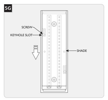
Align the large openings in the keyhole slots on the shade to the screws on the back plate and install the shade onto the backplate.
