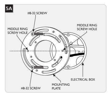
Align the two screw holes in the middle ring of the mounting plate horizontally and secure it to the electrical box with the two #8-32 screws provided.
