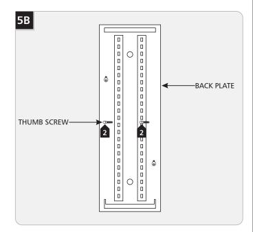
Temporarily mount the back plate onto the electrical 2 box using the thumb screws, mark the anchor hole locations, and remove the fixture.
