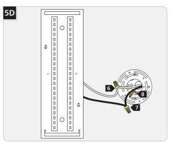
6 Connect the white fixture wire to the neutral power line wire with a wire nut.
