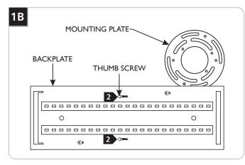
2 Unscrew the two thumb screws to separate the mounting plate from the backplate.
