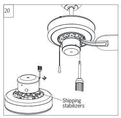
Remove shipping stabilizers from motor assembly.
