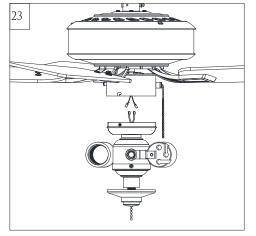
Connect light lead wires. White to white, blue (or black) to black (or blue). Make sure the quick connectors are clasped firmly.
