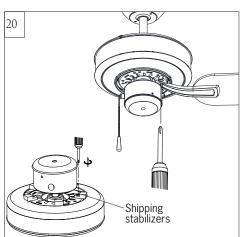
Remove shipping stabilizers from motor assembly.
