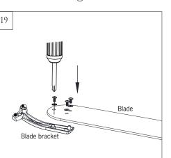
Install blade bracket with blade by 3 blade screws and washers provided. Tighten screws securely. Repeat this process for remaining blades.
