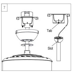
Install ball end of downrod into mounting bracket opening. Align (engage) slot on ball with tab on mounting bracket. **Warning:** Failure to align slot on ball with tab may result in serious injury. **Important**: If using the angle mount, make sure open end of mounting bracket is installed facing the higher point of the ceiling and make sure the ceiling angle is not steeper than 20°.
