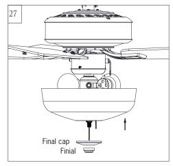
Align hole in center of final cap with thread rod, allowing pull chains to come through appropriate holes in the final cap, and push up. Thread center pull chain through hole in finial and secure glass to light fixture by tightening the finial. DO NOT OVER TIGHTEN the finial as glass may crack or break.
