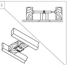
Before installing this fan make sure the outlet box is properly installed to the house structure. To reduce the risk of fire, electric shock, or personal injury, mount to outlet box or supporting system acceptable for fan support. (Mounting must support at least 35 lbs.)
