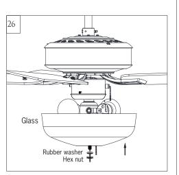
Raise glass in order to guide pull chains through appropriate holes in glass, aligning threaded rod on light fixture with hole in middle of the glass and push up gently allowing threaded rod to come through hole. (**Note**: Be sure pull chain for fan operation does not rub against bulb during operation).
