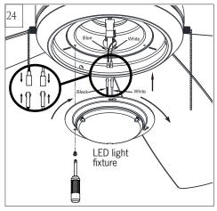
Connect white wire from fan to white wire from LED light fixture and then connect blue (or black) wire from fan to black (or blue) wire from LED light fixture.
