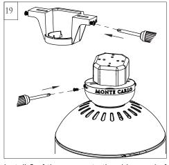
Install 2 of the screws to the side panel of mounting bracket corresponding to the open slotted holes on the canopy upper rim, screws provided. Remove the thread studs from the lower part of the mounting bracket.
