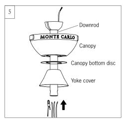
Place downrod over canopy, canopy bottom disc and yoke cover. Thread lead wires and safety cable from motor assembly through downrod.
