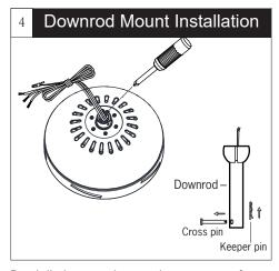
Partially loosen downrod set screws from yoke at top of motor assembly. Remove preassembled cross pin and keeper pin from downrod. Save parts.
