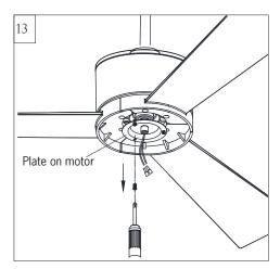
Loosen 2 and remove 1 preassembled screw from the plate on motor. Save screw for later use.
