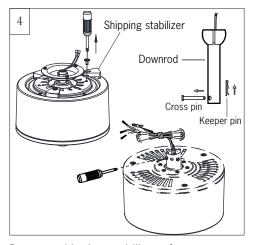
Remove shipping stabilizers from motor. Partially loosen downrod set screws from yoke at top of motor assembly. Remove preassembled cross pin and keeper pin from downrod.
