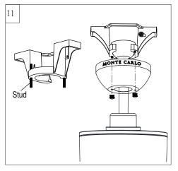
Lift Canopy, allowing the 2 studs to protrude through the canopy. Install knurled nuts provided and tighten the knurled nuts securely. The canopy should adjust for any irregularity in the ceiling or outlet box.
