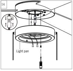
Connect the quick connector from fan to the quick connector from switch house (light pan). Be sure they are clasped together firmly.
