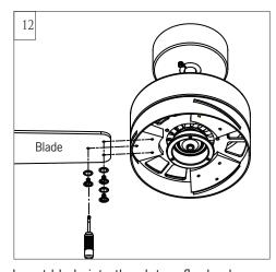
Insert blade into the slot on flywheel. Install blade with screws and fiber washers provided, aligning each of the holes as shown and tighten all screws securely. Repeat this process for remaining blades.
