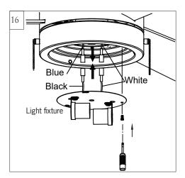
Connect white wire from fan to white wire from light fixture and then connect blue (or black) wire from fan to black (or blue) wire from light fixture.
