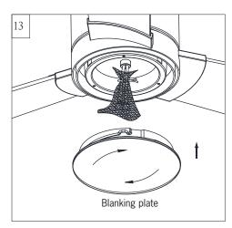
Attach a blanking plate by locating dimples in light pan with grooves on the blanking plate and twist clockwise until tight.
