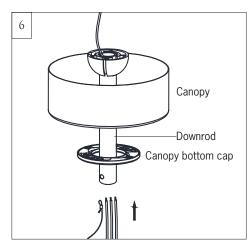
Place downrod over canopy and canopy bottom cap. Thread lead wires and safety cable from motor assembly through downrod.
