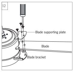
Install blade onto the blade bracket with a blade supporting plate as shown above by 3 blade screws provided. Tighten screws securely. Repeat this process for remaining blades.
