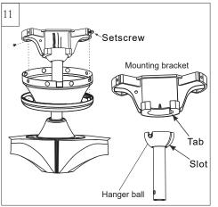
Install ball end of downrod into mounting bracket opening. Align (engage) slot on ball with tab on mounting bracket. **Warning:** Failure to align slot on ball with tab may result in serious injury. **Important**: If using the angle mount, make sure open end of mounting bracket is installed facing the higher point of the ceiling and make sure the ceiling angle is not steeper than 15°.
