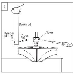
Flip the motor assembly with blades over. Partially loosen downrod set screws from yoke at top of motor assembly. Remove preassembled cross pin and keeper pin from downrod.
