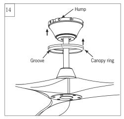
Raise canopy to mounting bracket, aligning loosened screws in mounting bracket with slotted holes in canopy. Twist canopy clockwise to lock. Reinstall screws (with washers) that were previously removed in step 3 and then tighten all screw securely Install canopy ring onto canopy by aligning the grooves in canopy ring with the humps on canopy and snap it onto canopy.
