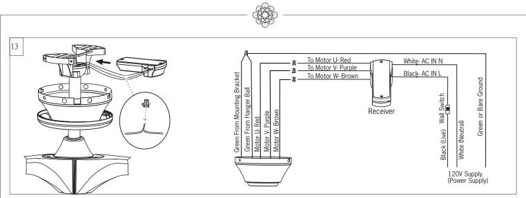
Make wiring connections using wire connectors provided as indicated above.
