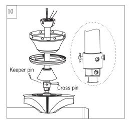
Slip downrod into motor yoke, aligning holes and install cross pin and keeper pin. Insert cross pin through yoke and downrod until point appears on the other side, and insert keeper pin on cross pin. Pull the downrod up tight against the cross pin, and then evenly tighten the downrod set screws on motor housing yoke.
