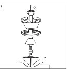
Thread lead wires and safety cable from motor assembly through downrod.
