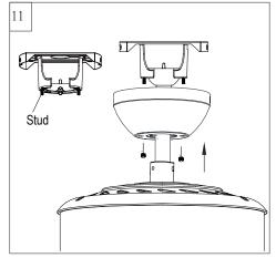
Lift Canopy allowing the 2 studs to protrude through the canopy. Install knurled nuts as shown. Tighten the knurled nuts securely. The canopy should adjust for any irregularity in the ceiling or Outlet box.
