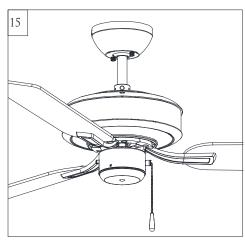
Install fan pull chains to preassembled pull chain on fan. Pull chain provided.
