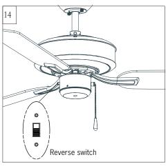
Setting the reverse switch in the down position will result in downward airflow and setting the switch in the up position will result in upward airflow.
