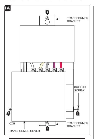
**NOTE:** In order to use small gage wires from the transformer to the electrical box, it is recommended to install the remote transformer near (if possible) the electrical box. See "Low Voltage Wire Size Table" below.
