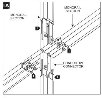
Push the four Monorail sections completely onto the three X conductive connectors.
