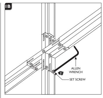
Tighten all the set screws with the Allen wrench provided. Make sure all set screw connections are tight for a proper power connection and to prevent heat build up.
