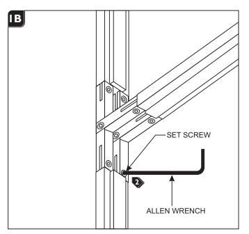
Tighten all the set screws with the Allen wrench provided.
