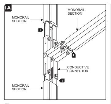
Push the three Monorail sections completely onto the two T conductive connectors
