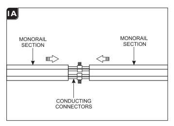
Push the two MonoRail sections completely onto the conducting connectors.
