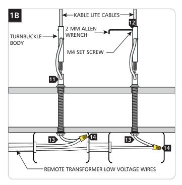
11 Feed the Kable Lite cables through the turnbuckle bodies into the post and through the threaded nipples into the electrical box(es).
