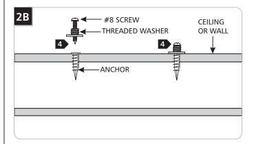
4 Attach the threaded washers to the anchors with the #8 screws.
