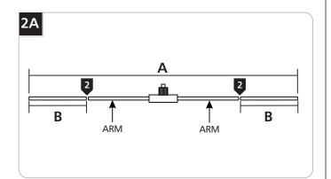
To cut the adjustable standoff arms refer to the chart above to determine the amount (B) that needs to be cut from each end.
