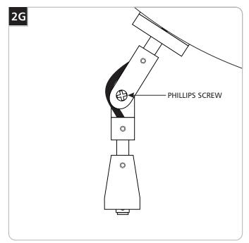
19 Ensure that the adapter is level and tighten the Phillips head screw.
