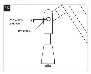
Tighten the set screw on the opposite side of the screw head with the provided .035 Allen wrench to ensure the position of the adapter.
