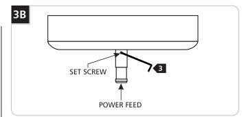
3 Loosen the set screw on the power feed.
