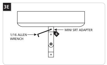
6 Install the Mini SRT adapter side of the power vault adapter assembly onto the canopy and tighten the #6-32 set screw with the 1/16 Allen wrench.
