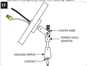
**12)** Loop the center wire and feed it completely through the second portion of the power vault adapter into the canopy.
