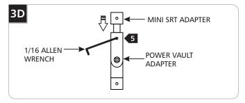
Install the Mini SRT adapter onto one end of the power vault adapter and tighten the #6-32 set screw with the 1/16 Allen wrench.
