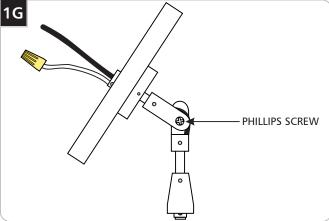
Ensure that the adapter is level and tighten the Phillips head screw.
