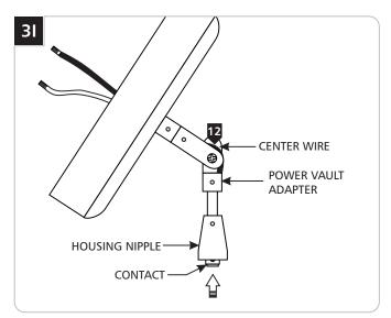
12 Loop the center wire and feed it completely through the second portion of the power vault adapter into the canopy.
