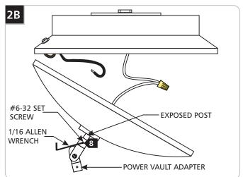
Push the power vault adapter completely onto the exposed post and tighten the #6-32 set screw with the 1/16 Allen wrench.
