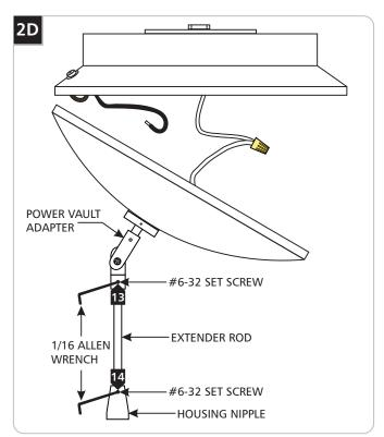
**NOTE:** The power extenders are precut for MonoRail power feed canopies. Power extenders must be cut to size when used with the surface mount transformers. Refer to the table below for the measurements.
