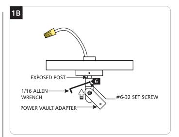
Push the power vault adapter completely onto the exposed post and tighten the #6-32 set screw with the 1/16 Allen wrench.
