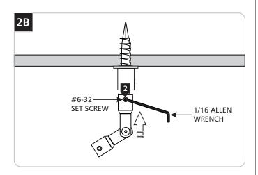
Push the vault standoff connector all the way onto the 1" joining rail and tighten the #6-32 set screw so that the connector is oriented in the proper direction.
