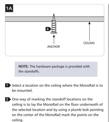
The other way is to hold the MonoRail directly against the ceiling and mark the standoff points on the ceiling.
