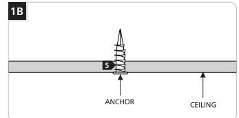
**5** Screw the anchors in the rest of the way with a Phillips screwdriver.
