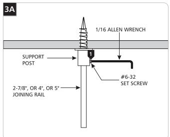
Insert the 2-7/8" joining rail (when 150 watt magnetic surface mount transformer is used with the system), or the 4" joining rail (when 300 watt magnetic surface mount transformer is used with the system), or 5" joining rail (when 600 watt magnetic or 300 watt electronic surface mount transformer is used with the system) all the way into the support post and tighten the #6-32 set screw with the 1/16 Allen wrench.
