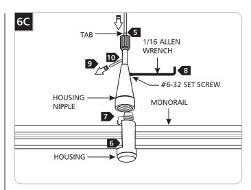
**5** Feed the aircraft cable through the wire grip by pushing the tab down. Pull the aircraft cable through the hole on the post.
