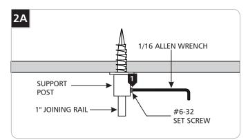
Insert the 1" Joining rail (provided with the vault adapter) all the way into the support post and tighten the #6-32 set screw with the 1/16 Allen wrench.
