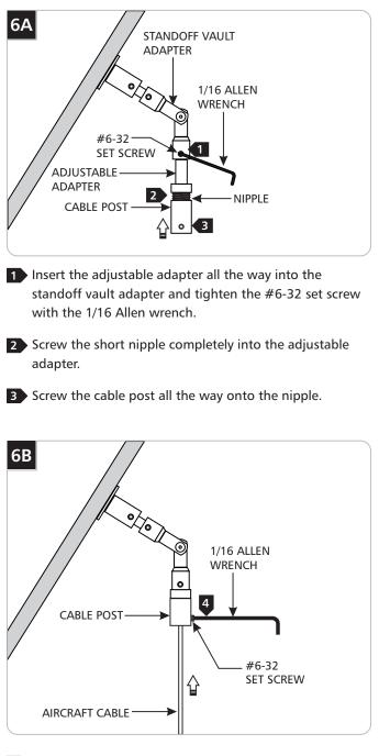
Insert the aircraft cable all the way into the cable post and tighten the #6-32 set screw with the 1/16 Allen wrench.
