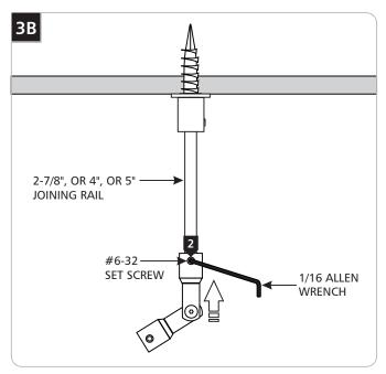
2 Push the vault standoff connector all the way onto the joining rail and tighten the #6-32 set screw so that the connector is oriented in the proper direction.
