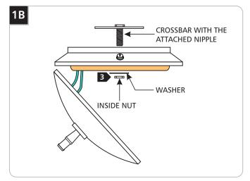
Remove the inside nut and washer to remove the crossbar with the attached nipple. **DO NOT REMOVE** the nipple from the crossbar.
