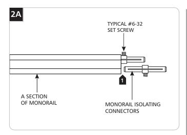
**NOTE:** Isolating connectors must be used inline with the MonoRail to isolate one transformer power feeds from the other.
