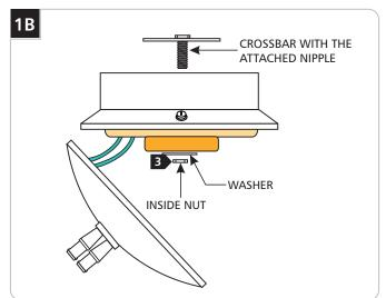
Remove the inside nut and washer to remove the crossbar with the attached nipple. **DO NOT REMOVE** the nipple from the crossbar.
