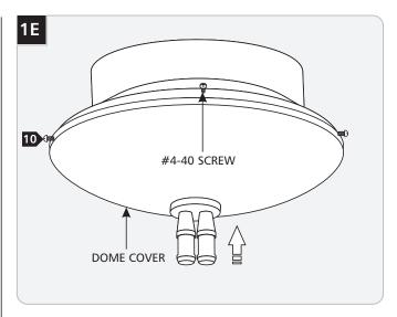
10 Replace the dome cover onto the transformer housing. Line up the dome cover holes with the transformer housing holes. Replace and tighten the #4-40 screws.
