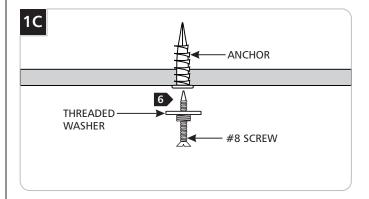
6 Attach the threaded washer to the anchor with the #8 screw.
