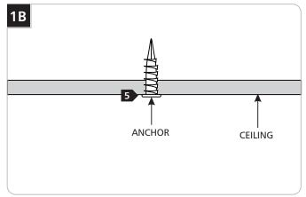
5 Screw the anchors in the rest of the way with a Phillips screwdriver.
