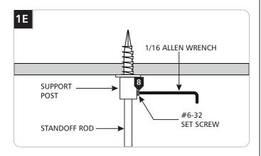
Push the standoff rod all the way into the support post and tighten the #6-32 set screw with 1/16 Allen wrench.
